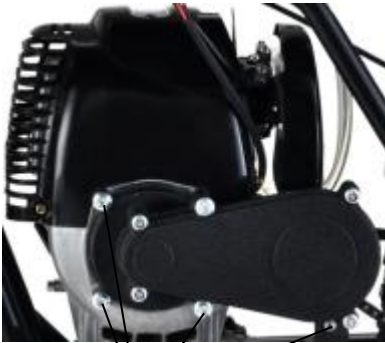
Loose 5pcs screws to take down gearbox
